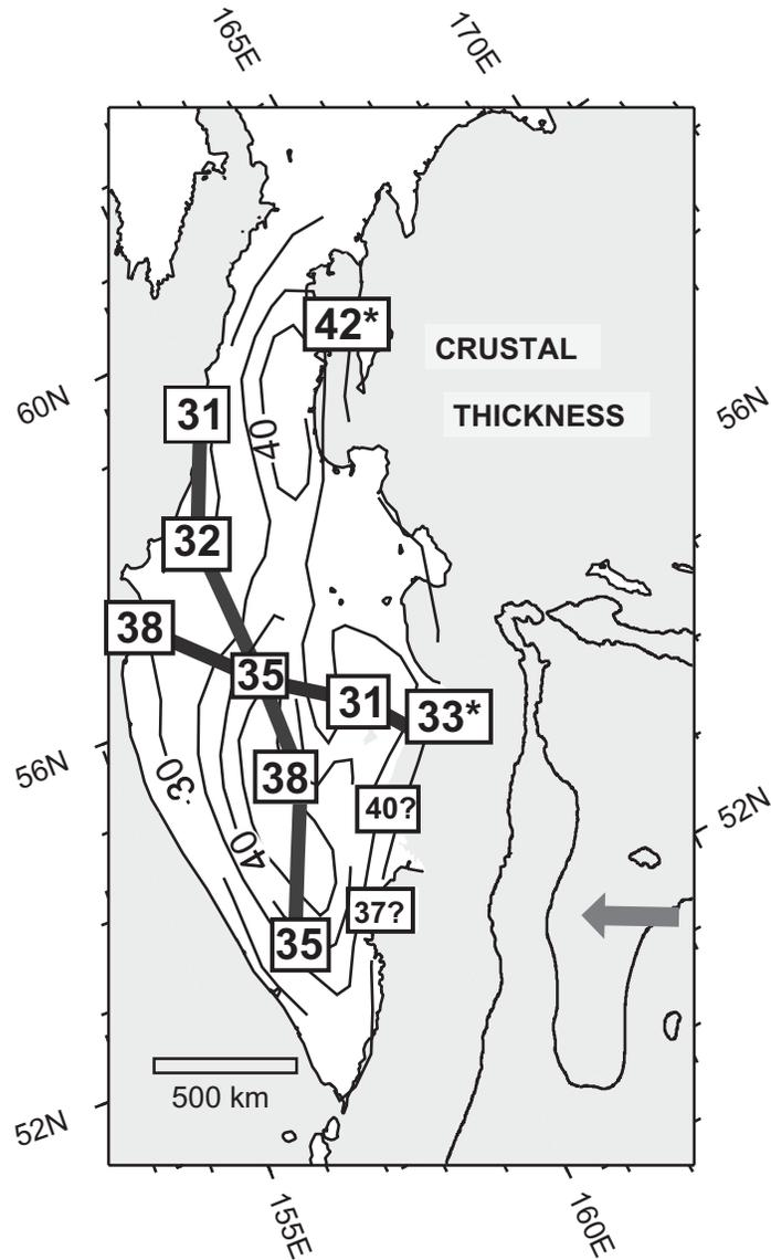
**Figure 10.** Crustal thickness map of Kamchatka generated by receiver function analysis of distant earthquakes (Levin et al., 2001). Individual thickness measurements are given in black boxes. Crustal thickness contours are from Bogdanov and Khain (2000). The deeply exhumed rocks of the Sredinniy Range occur in the region of the thickest crust of the Kamchatka Peninsula.
